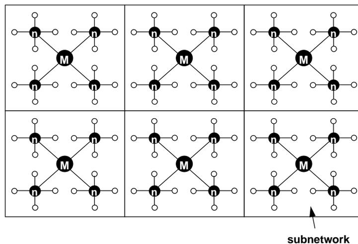
**Figure 5: Partially distributed master clocks network synchronization**
