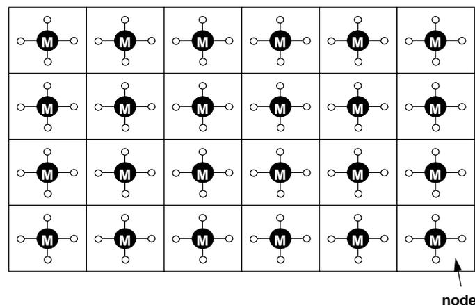
**Figure 3: Fully distributed master clocks network synchronization**
