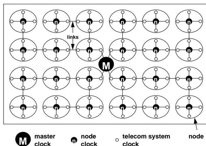
Figure 2: Centralized master clock network synchronization
